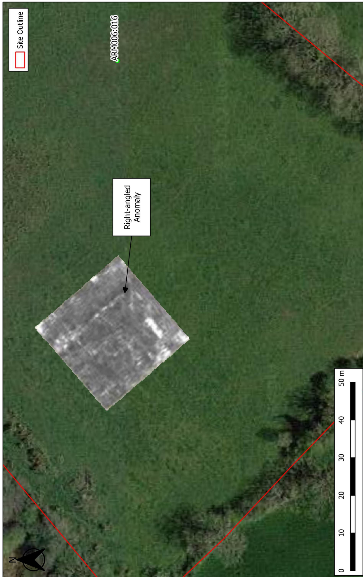
Figure 6: GPR Survey data showing 'Right angled anomaly'
