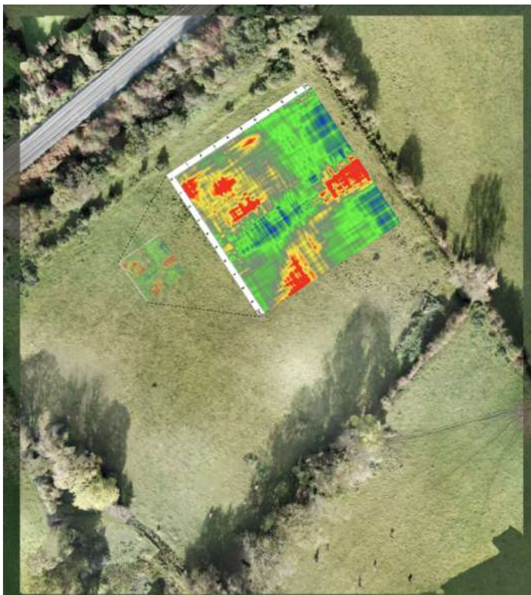
Figure 7. Detail of the Phase One 10 m x 10 m 3D survey (slice through the ground at 80 cm depth), same grid faded and overlain onto October 2021 drone orthoimage.
