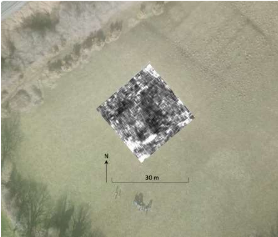
Figure 9. Greyscale 30 m x 30 m 3D slice at 1.35 m depth of the Phase 2 survey, overlain on March 1 st drone flight orthoimage.
