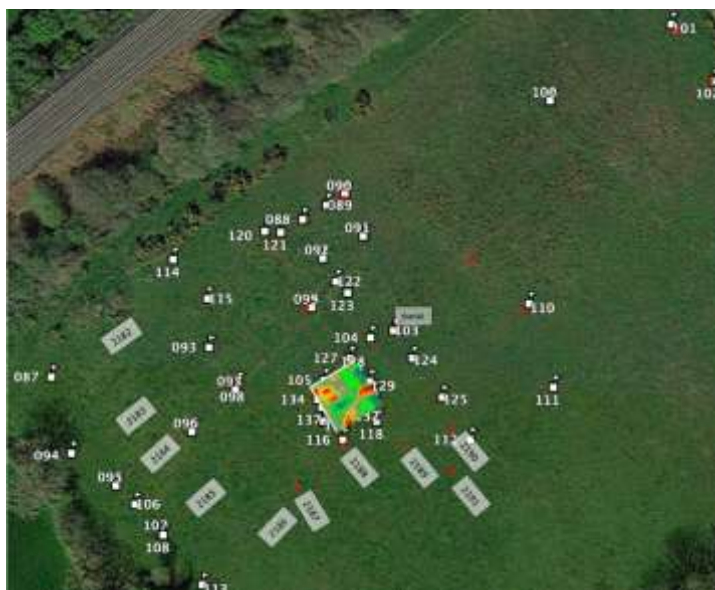
Figure 4. Reconnaissance GPR lines (red dashes), with Phase One 3D grid (coloured box). Numbers are GPS waypoints of 2D start and end points, plus anomalies noted in real-time. On GoogleEarth® aerial view.
