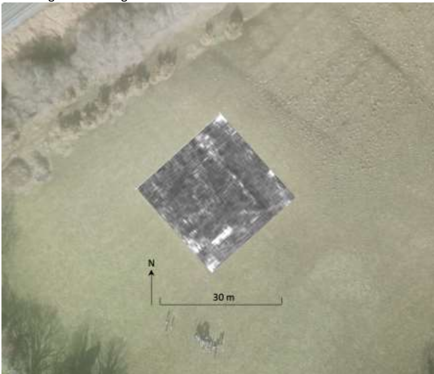
Figure 10. Greyscale radar amplitude 30 m x 30 m 3D slice at 1.35 m depth of the Phase 2 survey, overlain on March 1 st drone flight orthoimage.
